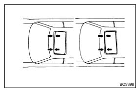
4. ADJUST CLEARANCE (Difference in left and right clearance)
