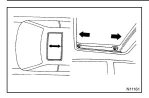
Adjust by loosening the sliding roof installation nuts and readjust the sliding roof to the proper position.
