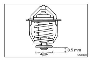
(c) Check that the valve is fully closed when the thermostat is at low temperatures (below 40°C (104°F)).
