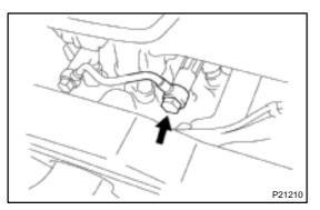
(d) Remove the union bolt holding the fuel pipe to the delivery pipe and gasket.
