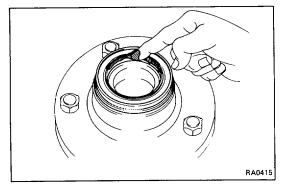
(c) Apply MP grease to the oil seal lip.
