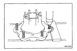
(e) Using a press, press in a new hub bolt.
