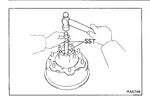
(b) Using SST, carefully tap in a new bearing outer race.
