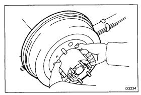
(c) Snug down the bearing by turning the hub several times.
