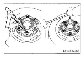
(c) Unstake the bolt and remove the nut.
