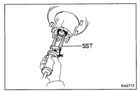
INSPECT OIL SEAL FOR WEAR OR DAMAGE If the oil seal is damaged or worn, replace it.
