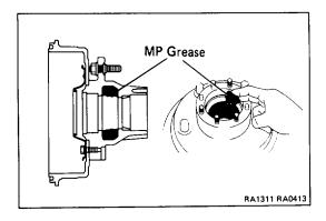
2. COAT SIDE HUB WITH MP GREASE
