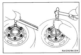
(f) Install and tighten the nut and stake the bolt.
