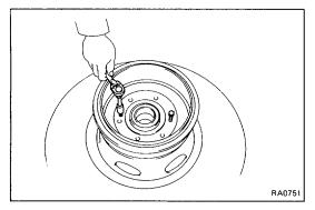
(b) Using the two service bolts, separate the hub and brake drum.
