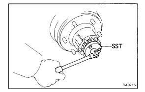
(b) Using SST, remove the bearing lock nut. SST 09509-25011
