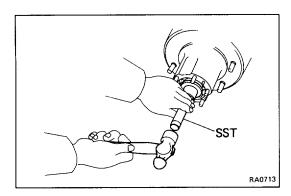
(b) Using SST, drive in the oil seal. SST 09517-12010
