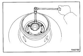
(g) Install the deflector and torque the six bolts.
