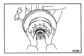
(d) Remove the hub and disc together with the outer bearing and thrust washer.
