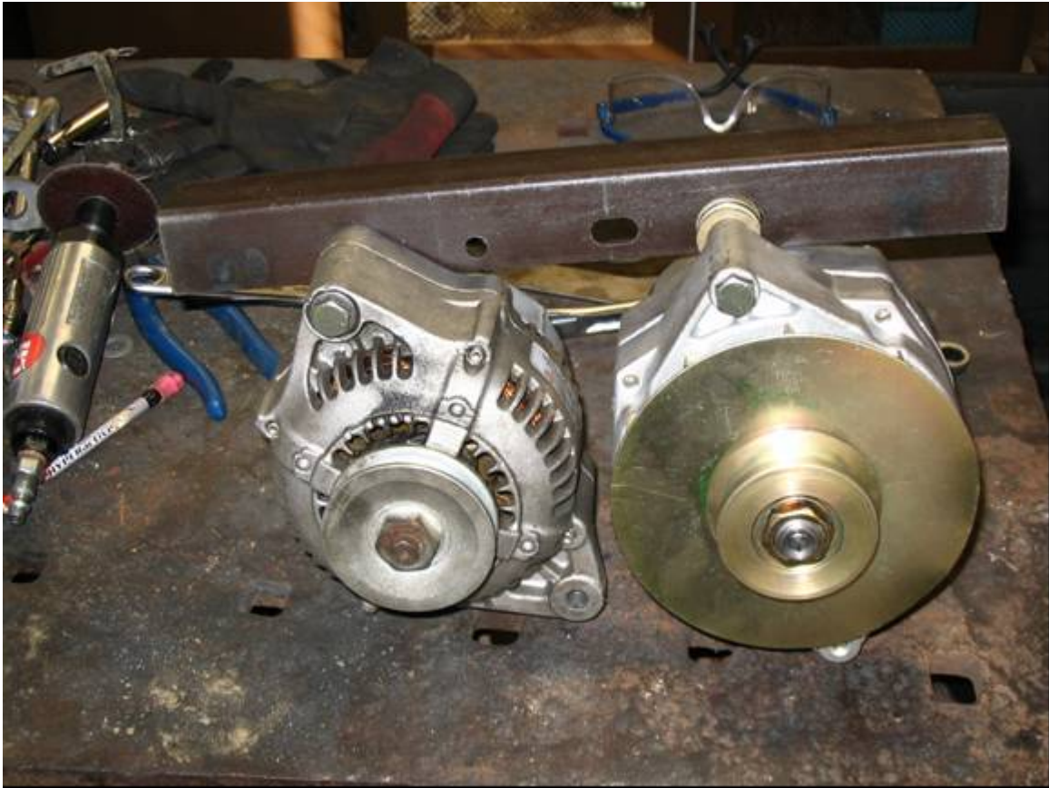
Figure 2. OEM alternator on the left; Powermaster PWM-47294 on the right. Note that the Powermaster is about \frac{1}{2} " larger diameter than OEM and location difference between the upper tabs (shown on the bottom of the alternators in this photo).
