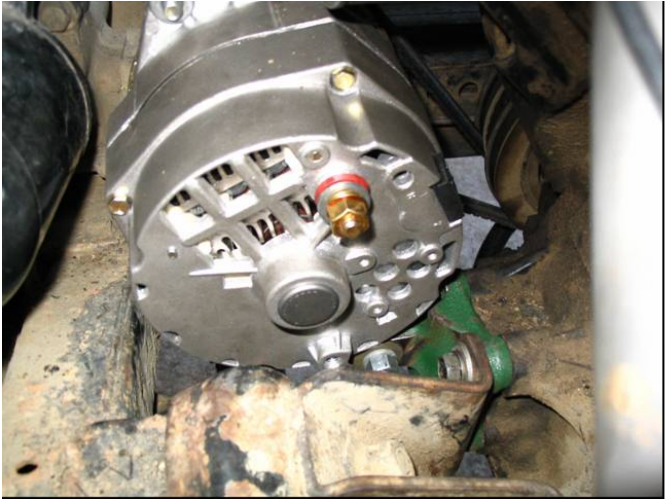
Figure 6. Powermaster PWM-47294 alternator installed and the belt tightened. Note the clearance between the alternator and the power steering cover on the left. Just barely visible in the extreme upper center is the upper radiator hose outlet. Although it's not clear from the photo, the alternator does clear the radiator outlet and hose. Note the large gold battery connection and the black dust cover at the ~2 o'clock position covering the #1 and #2 field and sensing connections respectively. The threaded hole just visible at the bottom of the alternator is for another mounting configuration, not for grounding.
