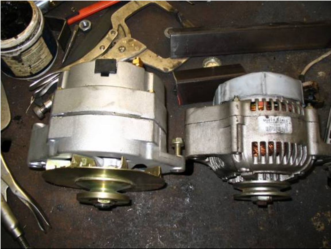
Figure 1. OEM Toyota alternator (Lester P/N 14668) on the right; Powermaster PWM-47294 GM 10SI 140 amp alternator of the left. Note the pulleys are almost lined up and the difference in mounting tab location, length and distance from the pulley.
