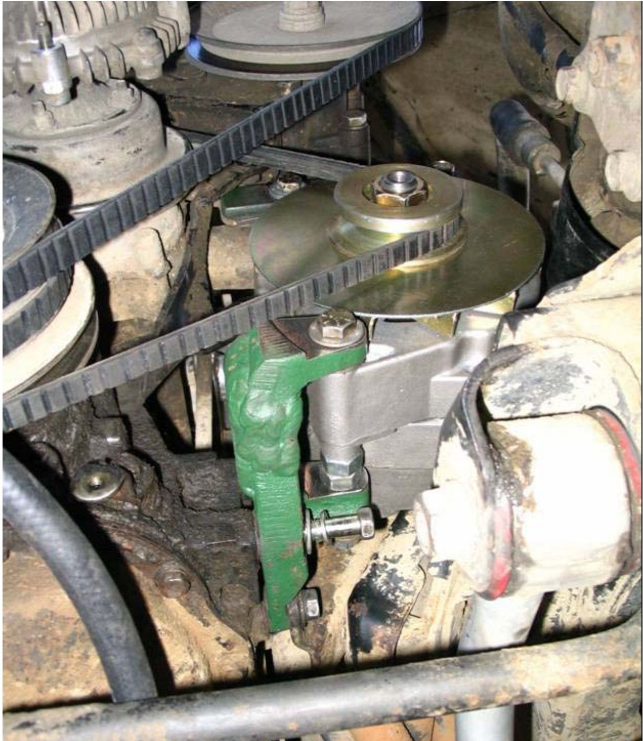
Figure 4. Lower mounting bracket cut, lengthened, rewelded and installed (in green).
