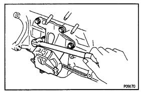
9. INSTALL LH AND RH ENGINE MOUNTING BRACKETS Install the mounting bracket with the 4 bolts. Install the 2 mounting brackets.
