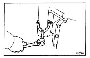
(e) Remove the 2 bolts, joint retainer, exhaust pipe and gasket from the catalytic converter.
