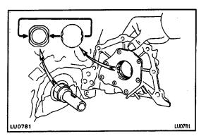
(d) Engage the spline teeth of the oil pump drive gear with the large teeth of the crankshaft, and slide the oil pump on the crankshaft.
