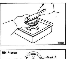
(c) Using solvent and a brush, thoroughly clean the piston. **NOTICE: Do not use a wire brush.**
