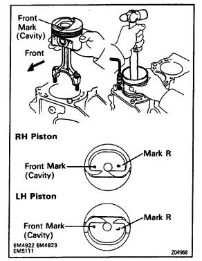
(b) Using a piston ring compressor, push the correctly numbered piston and connecting rod assemblies into each cylinder with the front mark of the piston facing forward.
