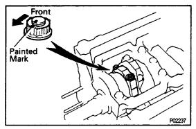
(c) Mark the front of the connecting rod cap nut and bolt with paint.
