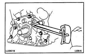
(e) Install the oil pump with the 8 bolts. Uniformly tighten the bolts in several passes.
