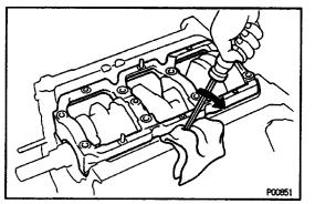
(b) Using a screwdriver, pry up the main beating cap, and remove the main bearing cap, lower main bearings and lower thrust washers (No.2 journal position of main bearing cap only).
