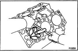
Using a cylinder gauge, measure the cylinder bore diameter at positions A, B and C in the thrust and axial directions.
