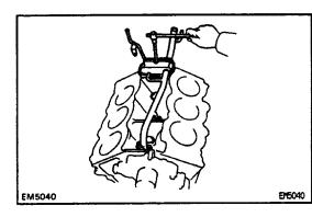
(c) Install the water bypass pipe with the 2 bolts and 2 nuts.
