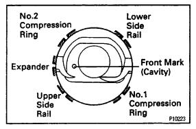
(b) Using a piston ring expander, install the 2 compression rings with the code marks facing upward. Code mark:
