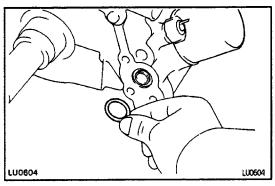
(b) Apply seal packing to the oil pump as shown in the illustration.
