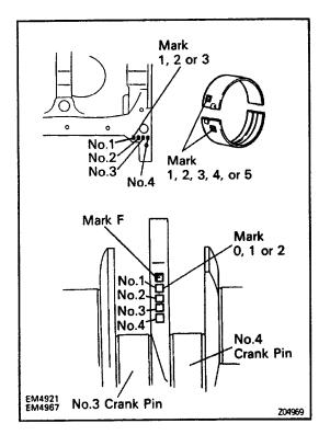
HINT: If using a standard bearing, replace with one having the same number. If the number of the bearing cannot be determined, select the correct bearing by adding together the numbers imprinted on the cylinder block and crankshaft, then selecting the bearing with the same number as the total. There are 5 sizes of standard bearings, marked "1 ", "2", "3", "4" and "5" accordingly.
