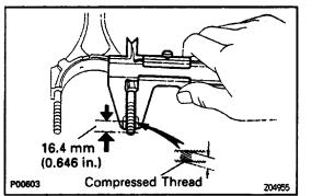
(b) If the cap nut cannot be turned easily, measure the outer diameter of the compressed thread with a vernier caliper. Standard outer diameter:
