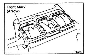
(b) Install the main bearing cap with the front mark facing forward.
