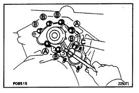
(b) Apply seal packing to the sealing groove of the water pump as shown in the illustration.
