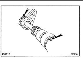
(c) Insert the distributor, aligning the groove of the distributor housing with the groove on the No.4 camshaft bearing cap.
