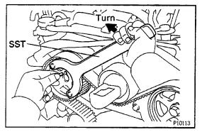
(e) Using SST, align the knock pin hole of the camshaft with the knock pin groove of the pulley and install the knock pin.
