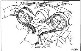
(b) Disconnect the timing belt from the camshaft timing pulleys.
