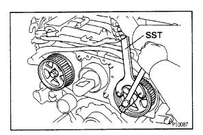
**20. REMOVE CAMSHAFT TIMING PULLEYS** Using SST, remove the pulley bolt, timing pulley and knock pin. Remove the two timing pulleys. SST 09278-54012
