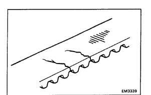
(c) If there is noticeable wear or cracks on the belt face; check to see if there are nicks on the side of the idle pulley lock.
