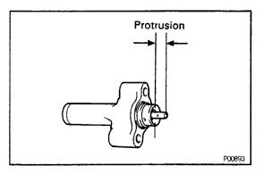
(c) Measure the protrusion of the push rod from the housing end.
