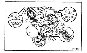
(b) Check that each pulley aligns with the timing marks as shown in the illustration.
