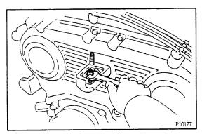
(b) Using the two water inlet nuts, remove the two stud bolts.
