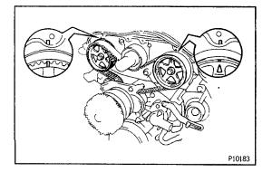
(b) Check that the timing marks of the camshaft timing pulleys and No.3 timing belt cover are aligned.
