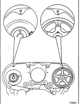
(b) (RH Camshaft Pulley Position)
