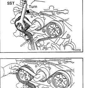
(a) Using SST, loosen the tension spring between the LH and RH camshaft timing pulleys by slightly turning the LH camshaft timing pulley clockwise.
