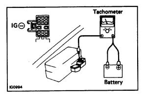
2. When a tachometer connected to the system, connect the tachometer test probe to the IGE) terminal of the DLC1.
