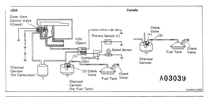
To reduce HC emissions, evaporated fuel from the fuel tank and float chamber is routed through the charcoal canister to the intake manifold for combustion in the cylinders.
