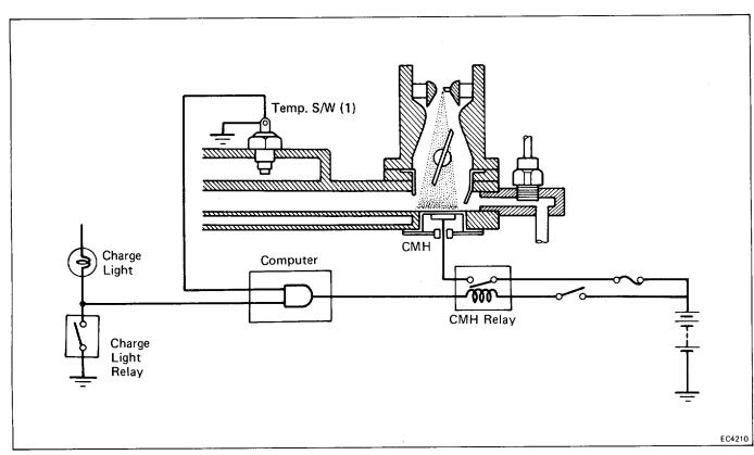
To reduce cold engine emission and improve drivability, the intake manifold riser is heated during cold engine operation to accelerate vaporization of the liquid fuel.
