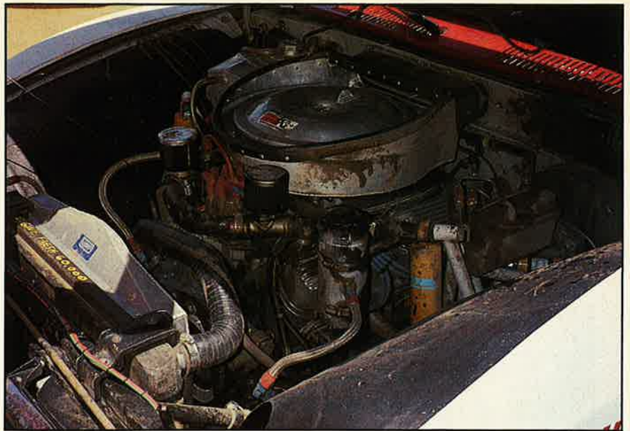
Stewart's 4Runner-bodied pre-runner has Ford V8, but one-seat race truck is all Toyota
