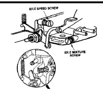
It is important to follow all linkage and lever installation instructions. The number one and two reasons for tuning errors are improper linkage installations and over tightened linkage nut, causing a binding in linkage assembly.
