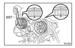
(c) Using SST, turn the camshaft pulley, align the timing marks of the timing pulley and No.3 timing belt cover. SST 09960-10010 (09962-01000, 09963-01000)
